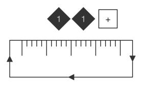
Fig. 12. Memory is implemented using recirculation of the impulses.
